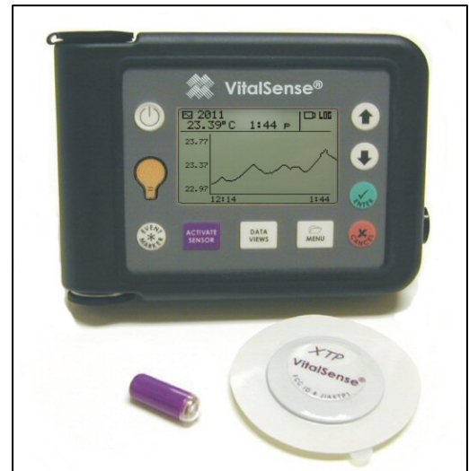
Wireless core and skin temperature measuring system used to monitor physiological parameters during training and competition.
